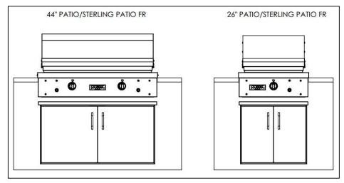
Clearance to Combustibles: Minimum clearance from either side of the grill (12") and the back of the grill (24") to combustible construction above the countertop must be observed. If the cabinet enclosure is constructed of combustible materials, the floor must be at least 25.5" below the bottom of the grill and the cabinet must be vented in 2 places, whether or not an LP tank is contained within (see Grill Enclosures Built With Combustible Material).
