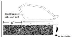
Hood Clearance: An 8" clearance is required behind the grill to allow the hood to open.
